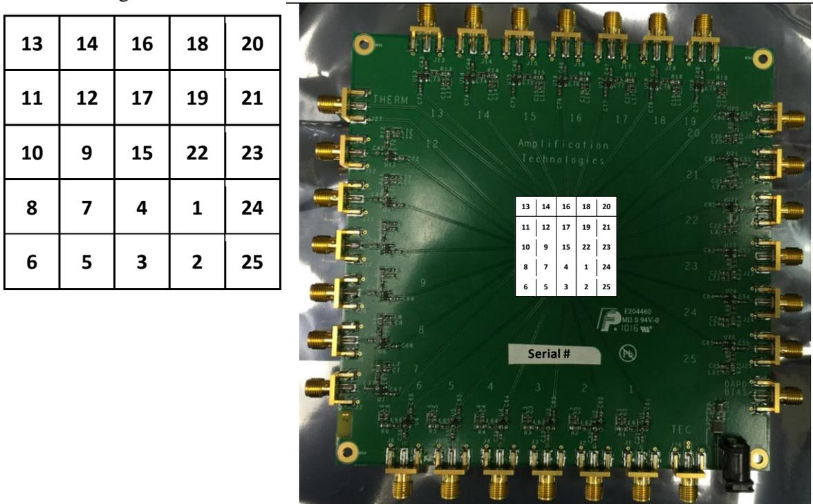
**Fig. 4:** Correlation between connector (pixel) IDs and array location
