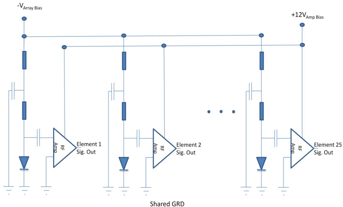
**Fig. 2:** Schematic connection diagram of the  $5 \times 5$  array and the 25 electronic pre-amplifiers network
