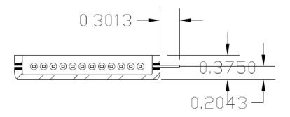
Note: The leads are delivered cut to 7.5mm (±1.5mm) length
